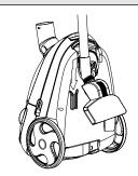
When storing the vacuum cleaner pipe and nozzle can be attached as shown in the picture.
